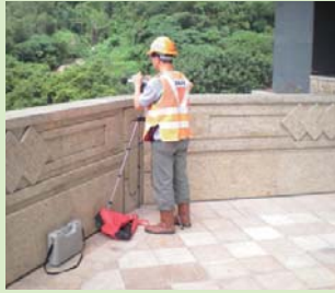
Regular noise monitoring in construction sites
