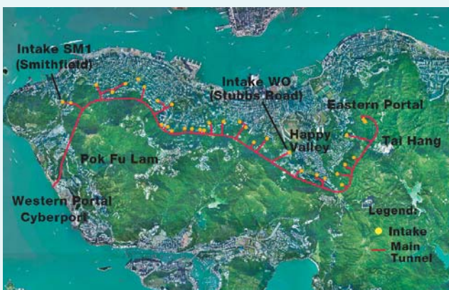
Locations of Eastern and Western Portals of Main Tunnel and Intakes that will be constructed soon
