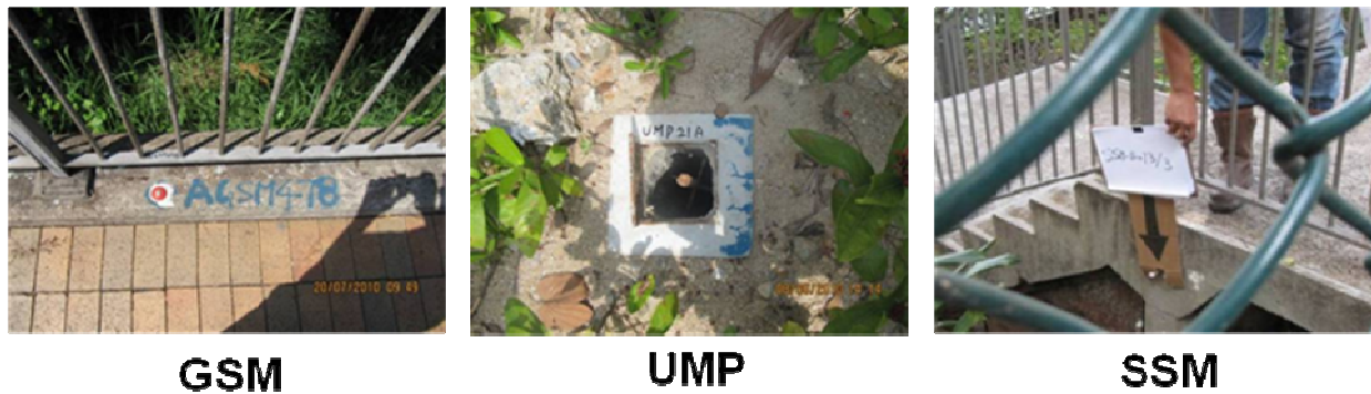
Figure 2 : Examples of Ground Settlement Marker (GSM), Utility Monitoring Point (UMP) and Structure Settlement Marker (SSM)
