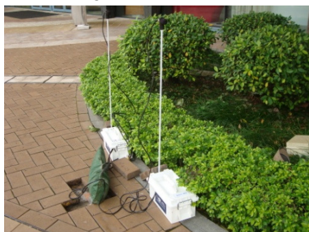
Plate 1 : Set-up of Seismograph Vibration Sensors and Air Overpressure Sensors
