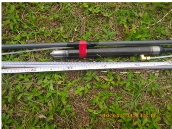
Plate 3 : Connect Borros type anchor to Rod Extensometer
