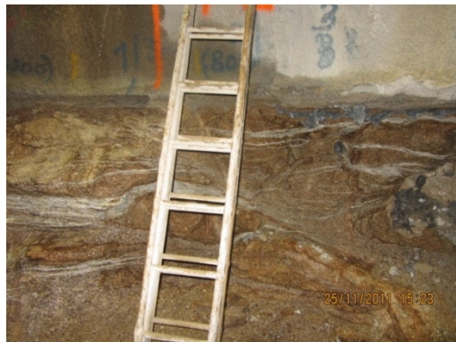
Plate 6 : Exposed Rockhead showing Presence of Micro-fines Cement Grout in Joints and Cracks
