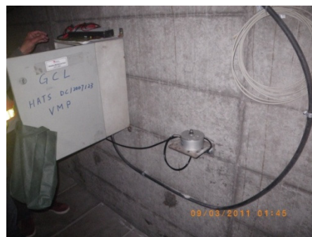
Plate 2 :Set-up of seismograph for real time vibration monitoring inside MTRC Tsuen Wan Line Tunnel
