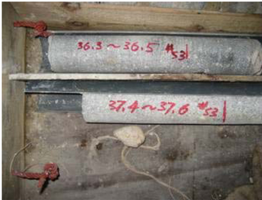
Photo 3: Core Sample of Jet-grouted Soil
