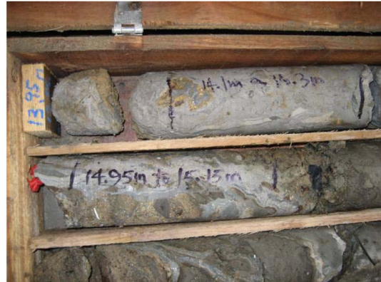
Photo 4: Core Sample of TAM-grouted Soil
