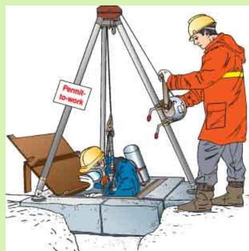
Worker wearing breathing apparatus and full-body safety harness with lanyard connected to a man-lifting tripod
