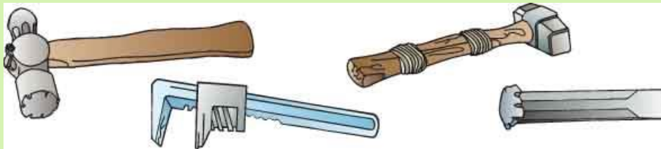
Defective hand tools
