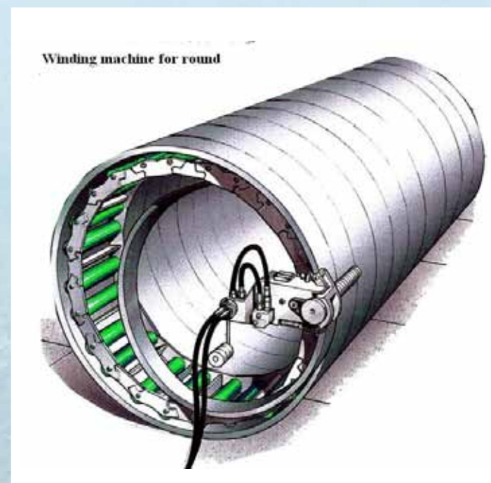
供大口徑管道用的繞線機 Winding machine for large diameter pipeline
